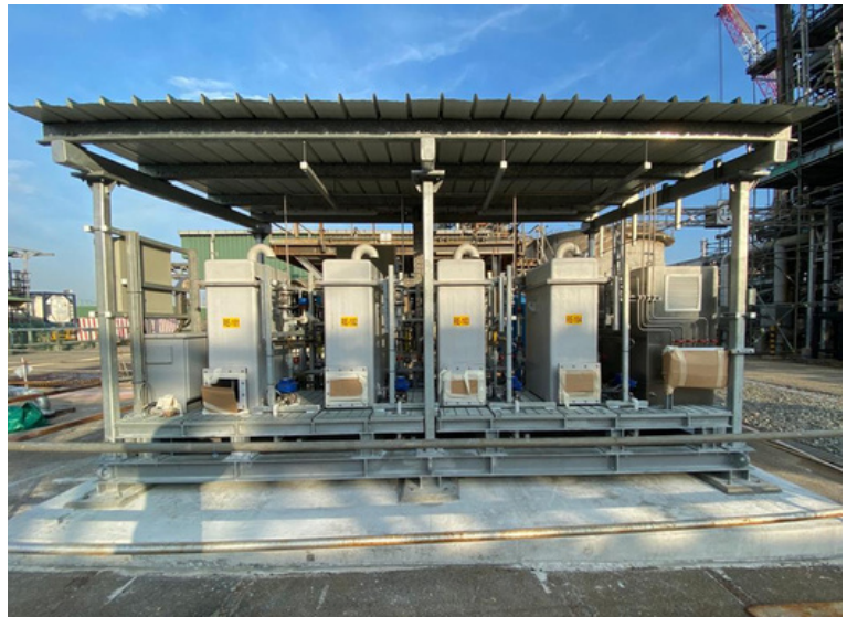
Left: Construction of AOP Skid in progress; Right: AOP Skid deployed at site
