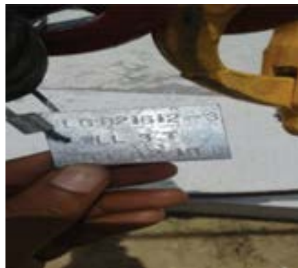
Ensure that the lifting gear tag number is correct.
